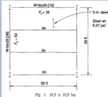
The cost of a filler beam and/or girder beam consists of the cost of the mill material, the cost of fabrication, and the cost of erection. The cost of fabrication and erection for a single beam is about the same for a heavy beam. Thus, beams should be spaced as far apart as practical to reduce the number of pieces that has to be made and erected on site.
