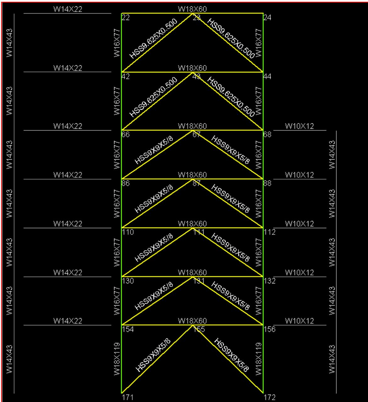
RAM Diagram: Section 1 7<sup>th</sup> Floor Plan
