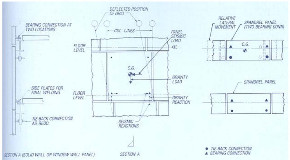
There is a problem however, with the connections of corner panels and connections. They must be designed to permit panels to slide past one another with minimum damage.
