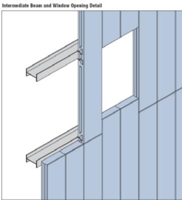
Seismic codes require that heavy panels accommodate movement either by sliding or ductile connections. In high seismic zones, sliding connections is not a good choice, because of the possibility of incorrect adjustments when bolts are used, jamming or binding due to unwanted materials left after installation and jamming due to geometrical change of the structural frame under horizontal forces.
