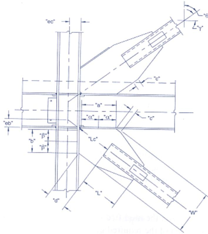
15.5 Brace-to-Beam Midspan Connection Diagram
