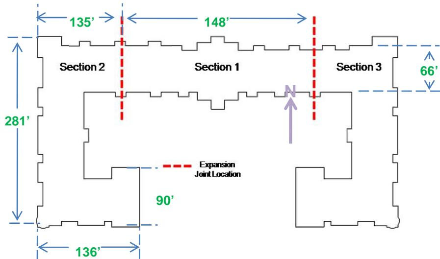
The relocation of expansion joints is needed due to the irregular configuration of the building. Two main problems related to seismic performance that may result are:
