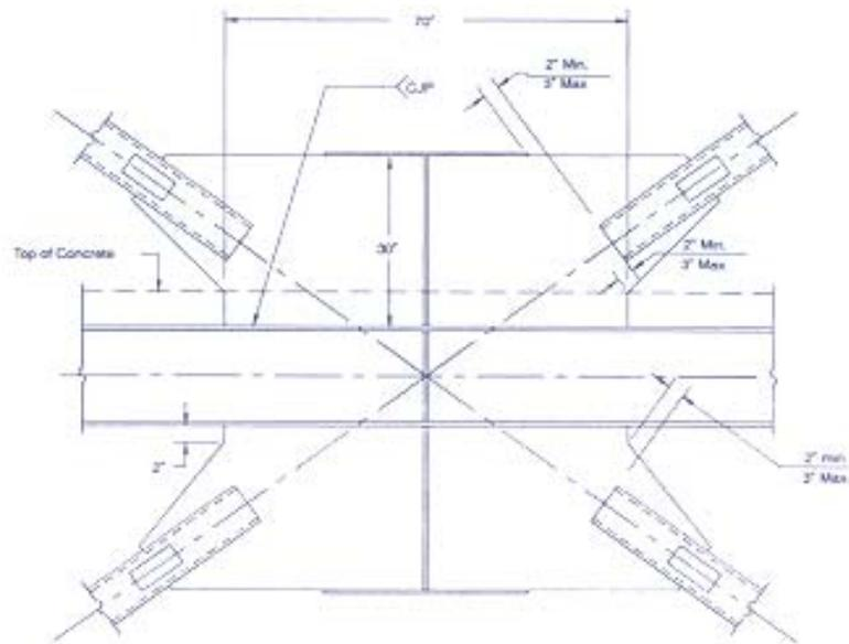
15.6 Brace-Beam-Column Connection Design
